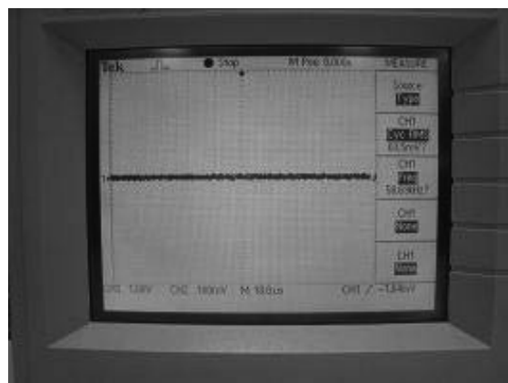
U9 Pin 4 –DAC_FLD (OSD Off), Idle
